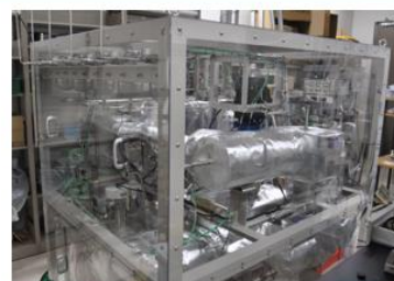
Above: FLiBe test loop benchtop experiment sited at Kyoto University (Inconel 600).
