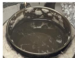
Below: melted FLiBe in a pot before purification.
